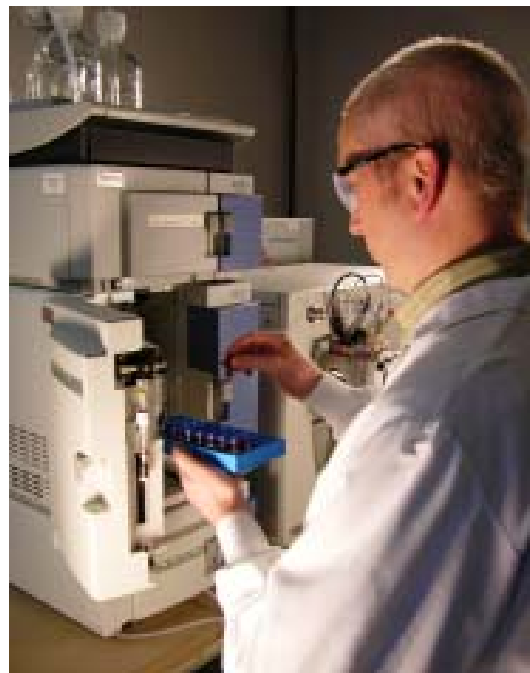
Dr. Robert Duff, manager of Biochemistry, works with Thermo Scientific LTQ XLTM Orbitrap Mass spectrometer to confirm oligonucleotide mass and sequence.
