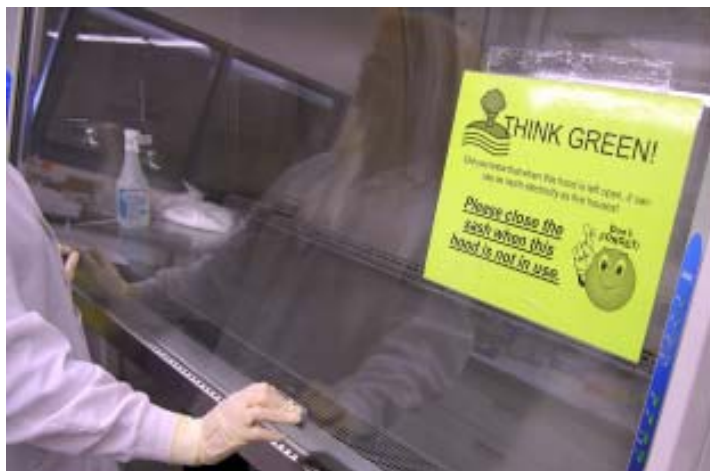
Keeping hood sashes closed while not in use results in significant cost savings in electricity/heating bills as well as reducing the amount of energy wasted when left open.
