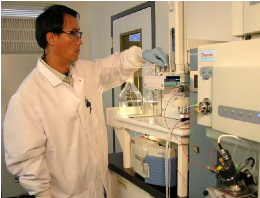
Dr. Xiaoping Xia, Method Development & Validation principal chemist, develops a method to determine the amount of melamine and cyanuric acid in raw materials, using a Thermo TSQ Vantage LC/MS/MS.
