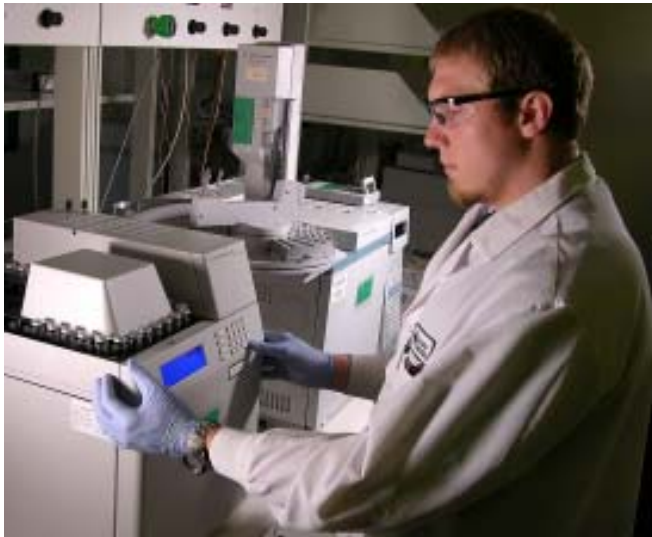
Wes Atkins, senior method validation chemist, performs residual solvent analysis by headspace GC.
